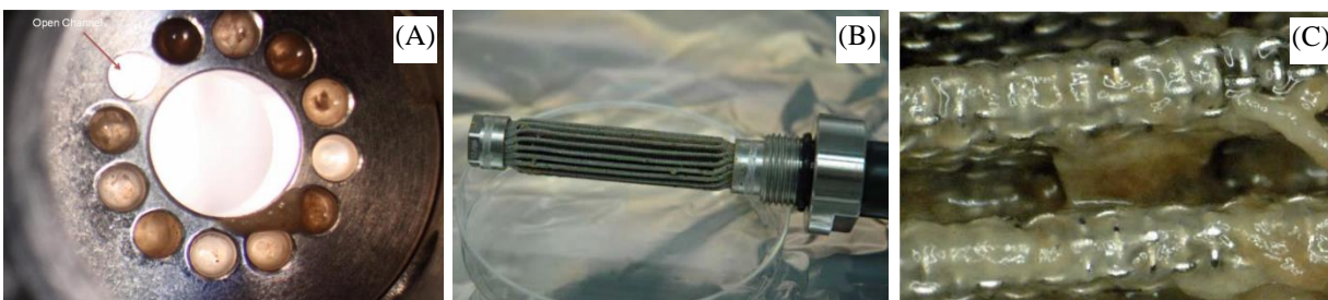
Figure 2. (A) Biofilm Present in the MLS inlet Solenoid Valve of the Pump/Sep ORU returned in 2010. 8 (B) The mesh filter in the EFA returned in 2011, and (C) a close-up of its inlet section. 9
