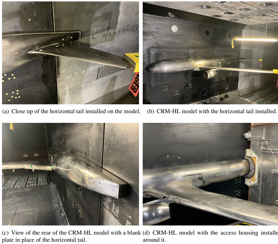
Fig. 16 Pictures of the horizontal tail installation on the NASA 5.2%-scale CRM-HL model [Photos: NASA].
