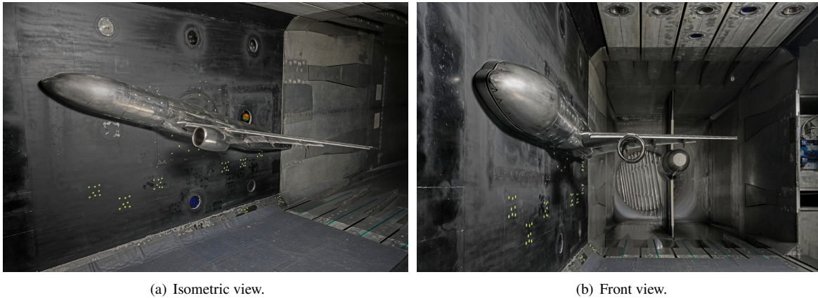
Fig. 1 Pictures of the NASA 5.2%-scale CRM-HL semispan model installed in the NTF [Photos: NASA].
