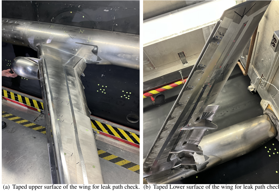
Fig. 34 Taping of the wing for leak path checks [Photos: NASA].
