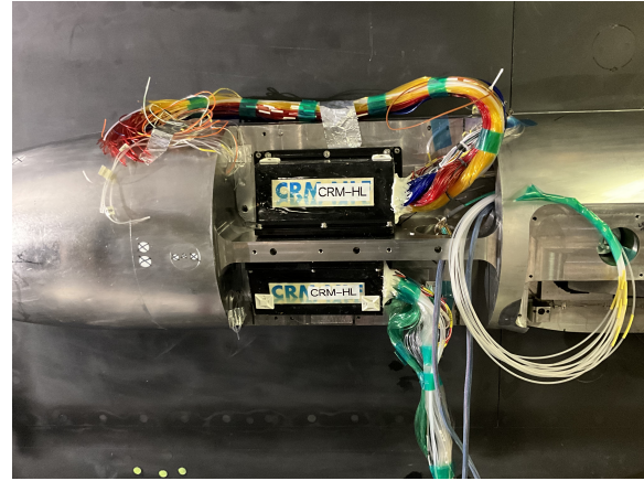
(b) Close up view of the ESP heater boxes in the fuselage, mid-installation.
