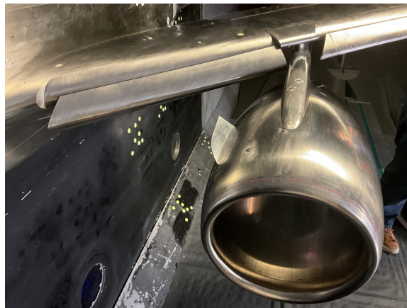
Fig. 12 Picture of the 5.2%-scale CRM-HL nacelle [Photo: NASA].
