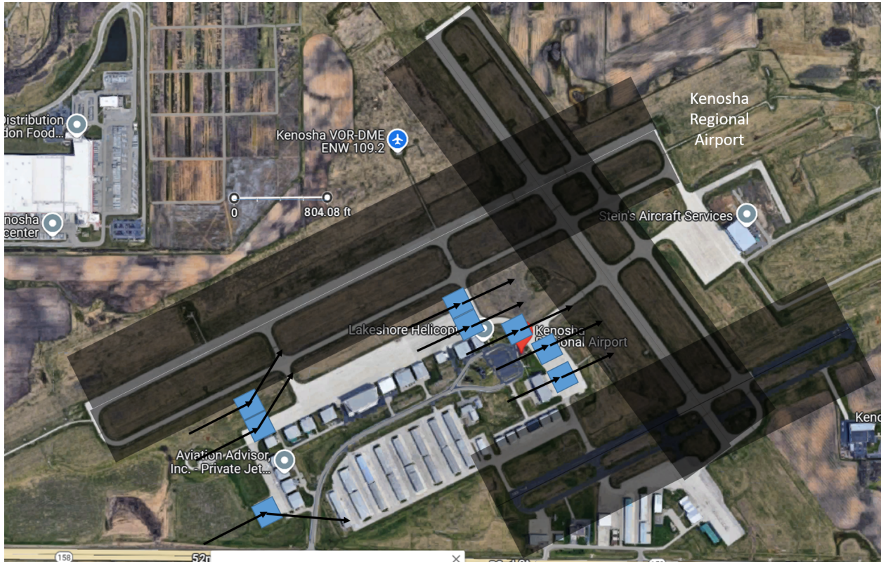
Fig. 18 TLOF pad locations for Kenosha Regional airport. The relatively low demand and large number of TLOF pads (eight), result in this aerodrome being relatively unaffected by throughput constraints. Maps data: Imagery ©2025 Google, Imagery ©2025 Airbus, Maxar Technologies, Map data ©2025
