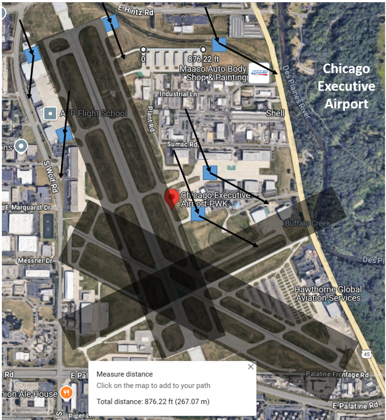
Fig. 15 Chicago Executive airport showing the location of six TLOF pads, each with independent approach and departure vectors. Maps data: Imagery ©2025 Google, Imagery ©2025 Airbus, Maxar Technologies, Map data ©2025
