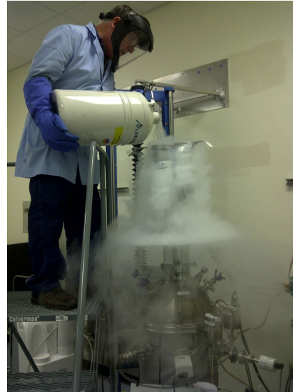
Figure 1. Cut-Away of CS-100 Assembly Showing Major Components/Details (left); CS-100 During LN 2 Fill Procedure (right)
