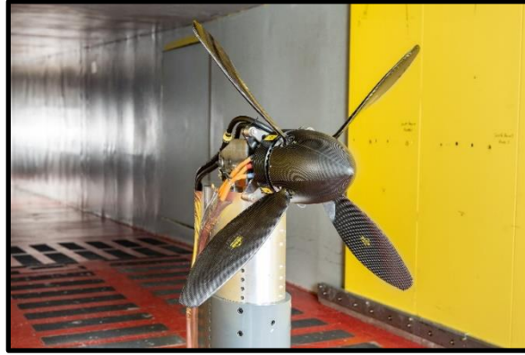
Fig. 1 NASA's eVTOL Propeller Test Stand for Fundamental Icing Physics Studies
