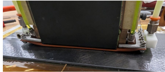
Figure 23. Induction welding pressure bladder
