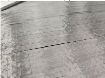
Figure 7. Tows not sticking because of roller bridging
