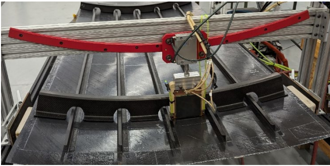
Figure 22. Induction welding of frames
