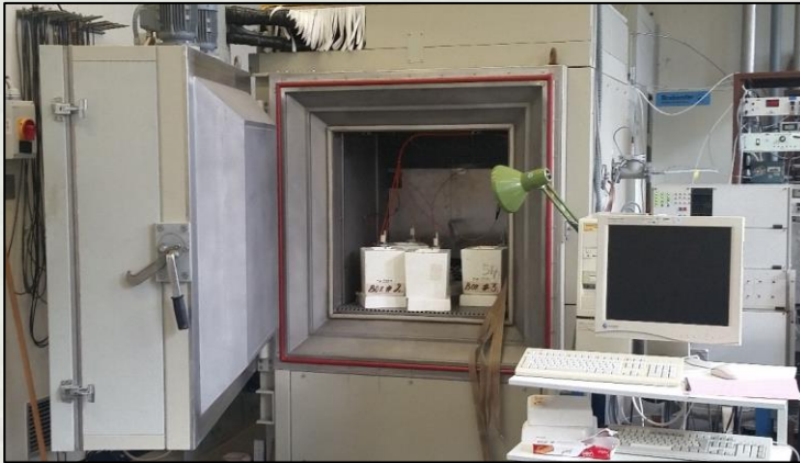
World Calibration Centre for OzoneSondes (WCCOS) environmental chamber
