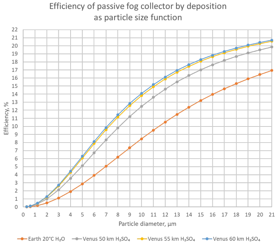
Figure 23. Collection efficiency of the fog harp collector. The x-axis is the particle diameter and the y-axis is the percentage efficiency of collection. The efficiency is higher for sulfuric acid droplets compared to water. We see that the collection efficiency increases for higher altitude due to lower temperature, which causes changes in viscosity.
