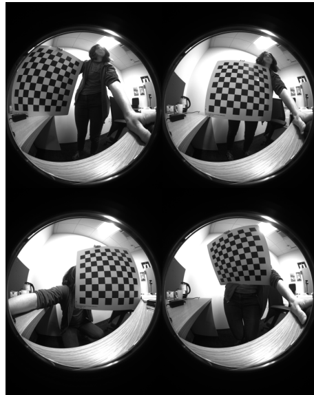
Figure 12: Mosaic of Fisheye Images Captured for Calibration.
