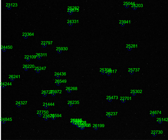
Figure 13: Uncalibrated Star Identification on ODIN NAC Image. Green Indicates Projected Stars with Hipparcos ID Label. Blue Circles Indicate Detected Star Centroids.
