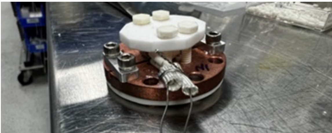
Figure 63. The prototype TEG device encapsulated in the jig.
