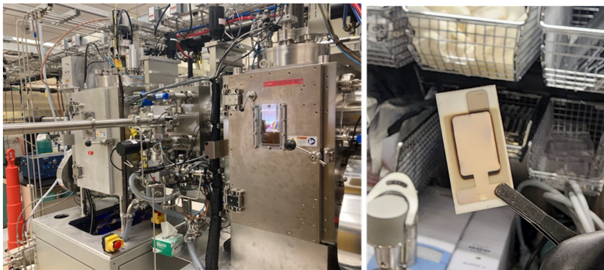
Figure 22. Image of ORNL Li deposition tool (left) and LMNO/LiPON/5 \mu\text{m} Li heterostructure after deposition (right).
