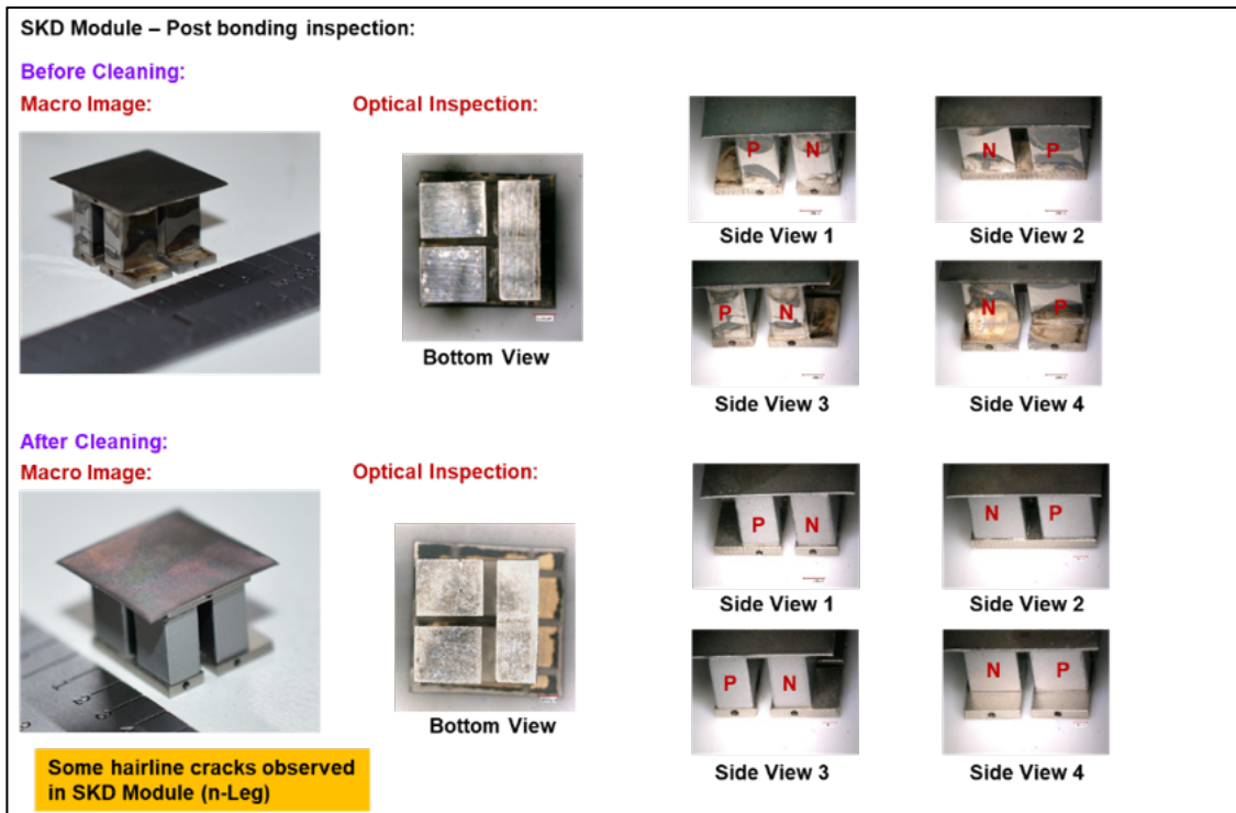
Figure 57. Skutterudite bi-couple #2 post bonding inspection.
