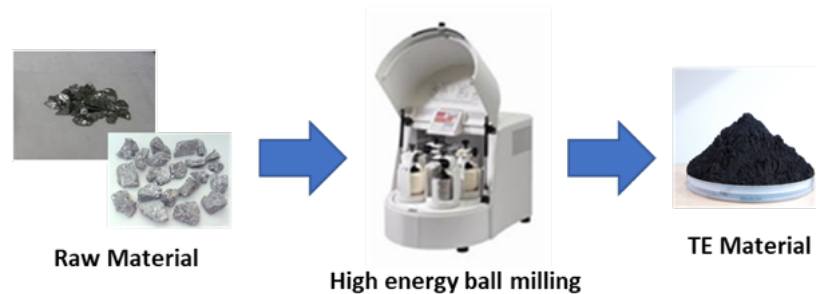
Figure 46. Ball milling was performed to make the SKD precursor materials.
