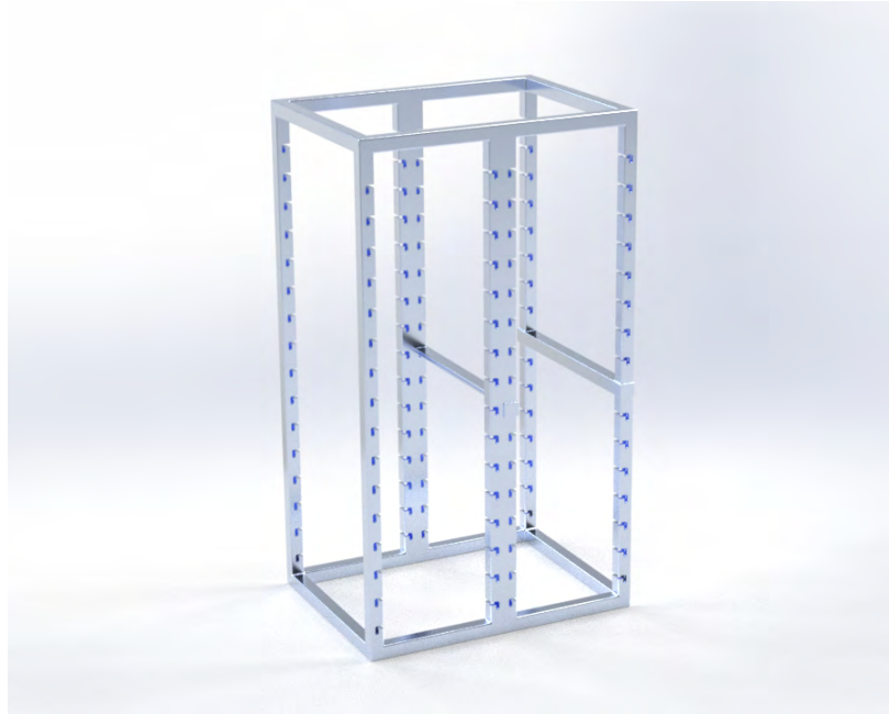
Figure 92: CAD Model of Notched Design for Payload Rail Integration
