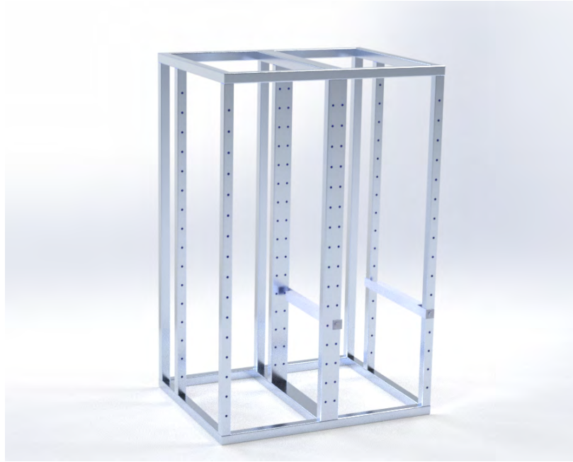
Figure 95: CAD Model of Bolted Design for Payload Rail Integration
