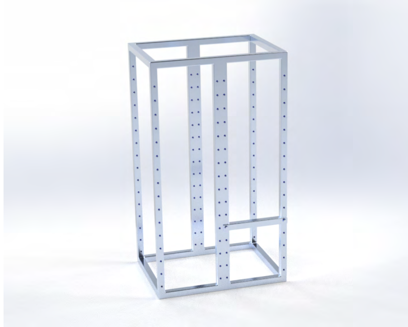
Figure 93: CAD Model of Bolted Design for Payload Rail Integration
