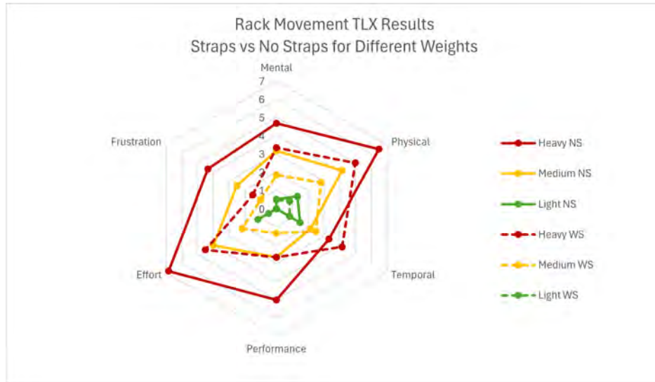
Figure 50: Dry Land Rack Movement TLX Results Averaged Across all Test Groups for Various Weights (Straps vs No Straps)
