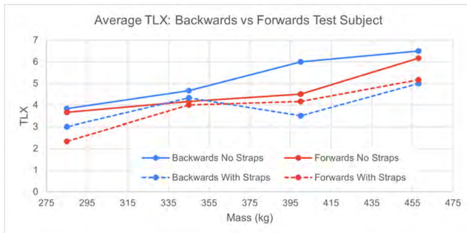
Figure 61: Underwater Testing Average TLX Data for Test Subjects Facing Backwards and Forwards (Straps vs No Straps)
