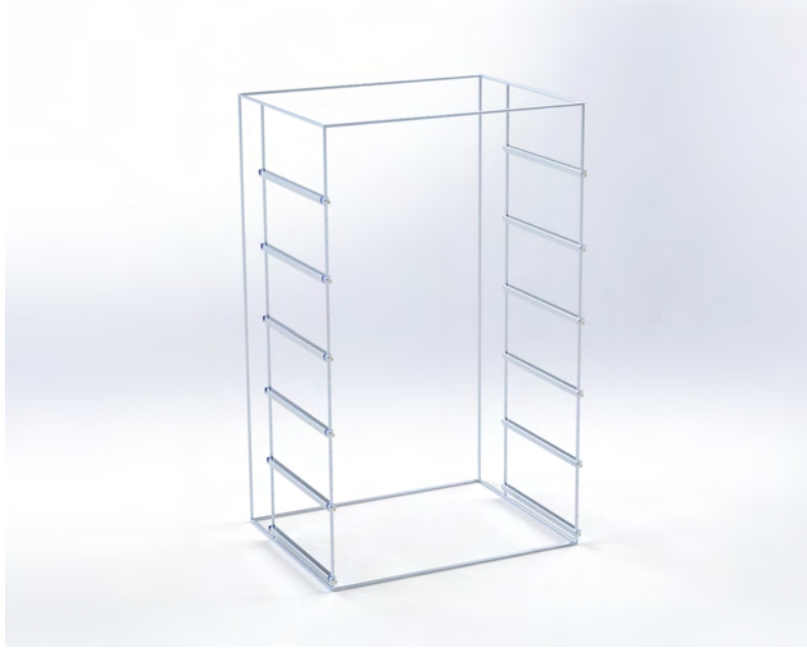
Figure 2: CAD Model of Double Rack Frame
