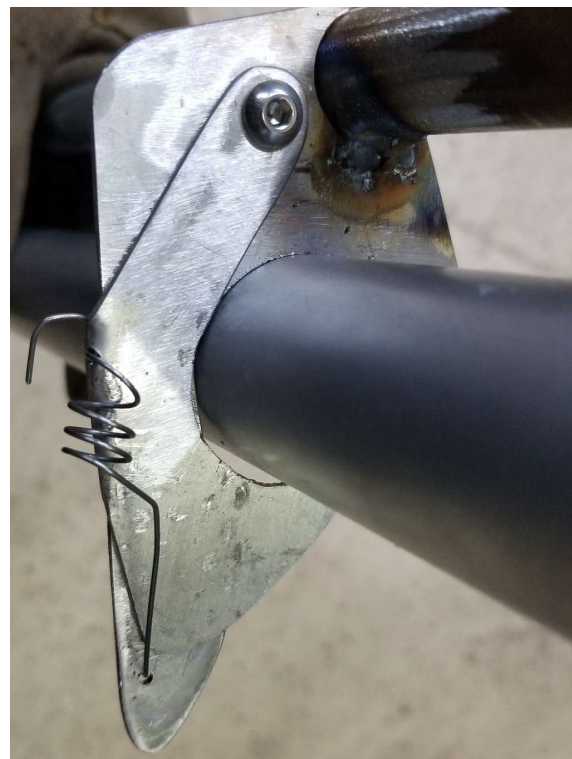
Welded steel prototype, which worked well, though it required quite a lot of hand welding.
