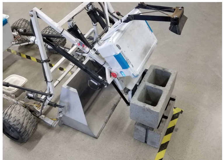
Full scale teleoperated test of our multipurpose robot stacking cinderblocks (17kg) with forklift-style forks.
