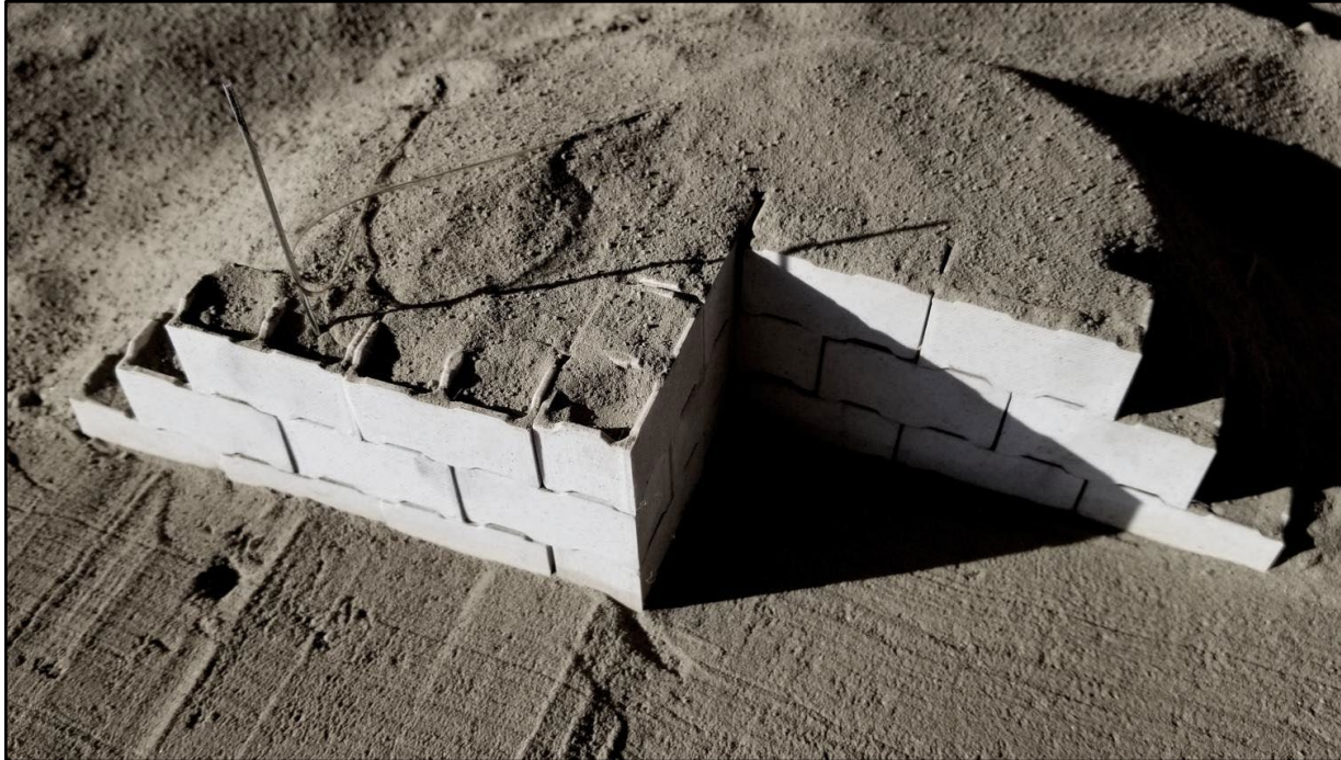
1/10 scale dry-stacked modular wall, assembled manually in fine basalt dust. Basalt fiber rods could act as continuous vertical rebar, and basalt fiber strands could tie the rebar back into the dust like a geotextile anchor (examples of both on left).
