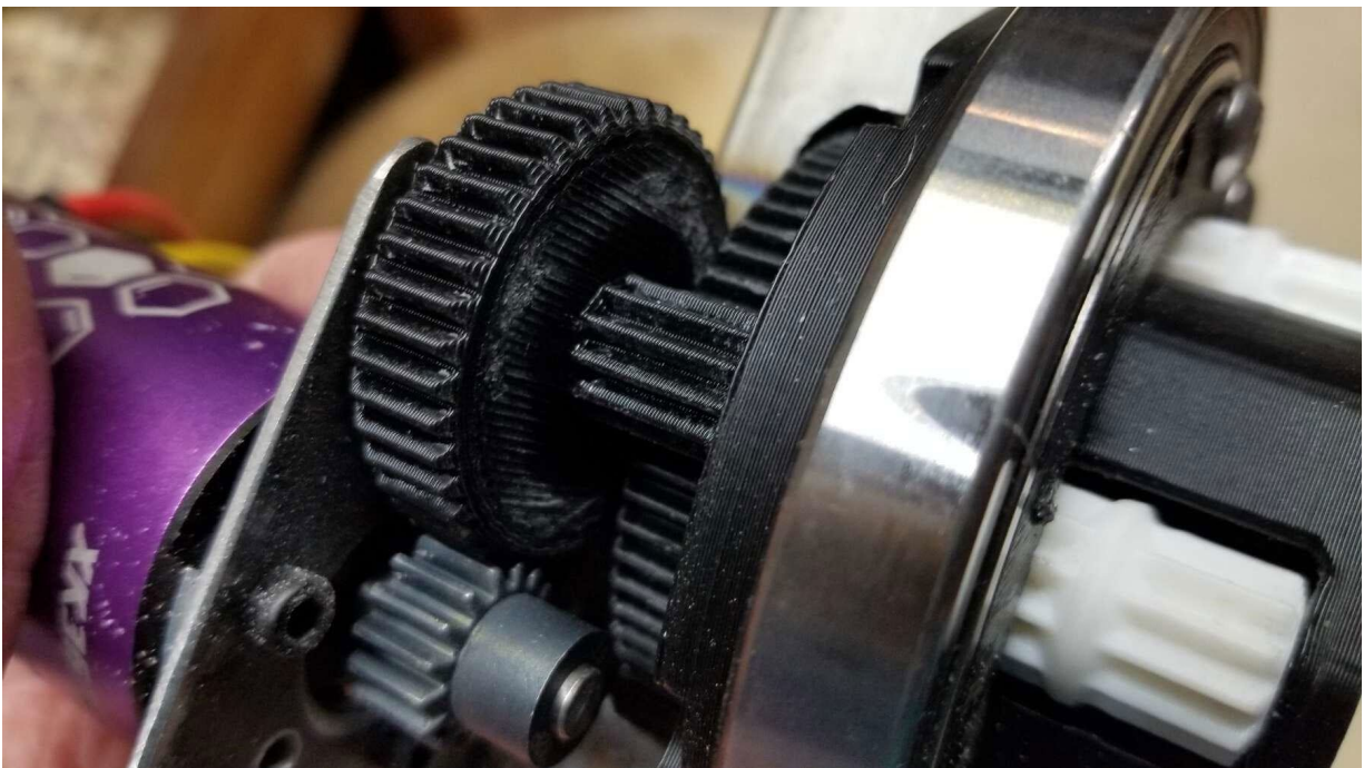
The brushless motor spins an intermediate reducer gear, which spins the sun gear, which drives the planets, which moves the arm.
