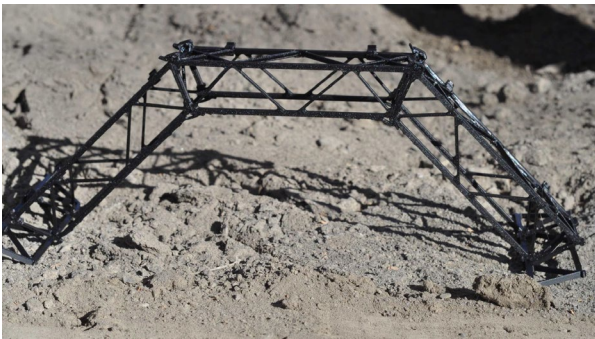
A 1-section 3-segment arch, with flat L-truss plates used as the crucial foundation element, in fluffy basalt rock crusher dust (NP-1, similar to BP-1 regolith simulant).
