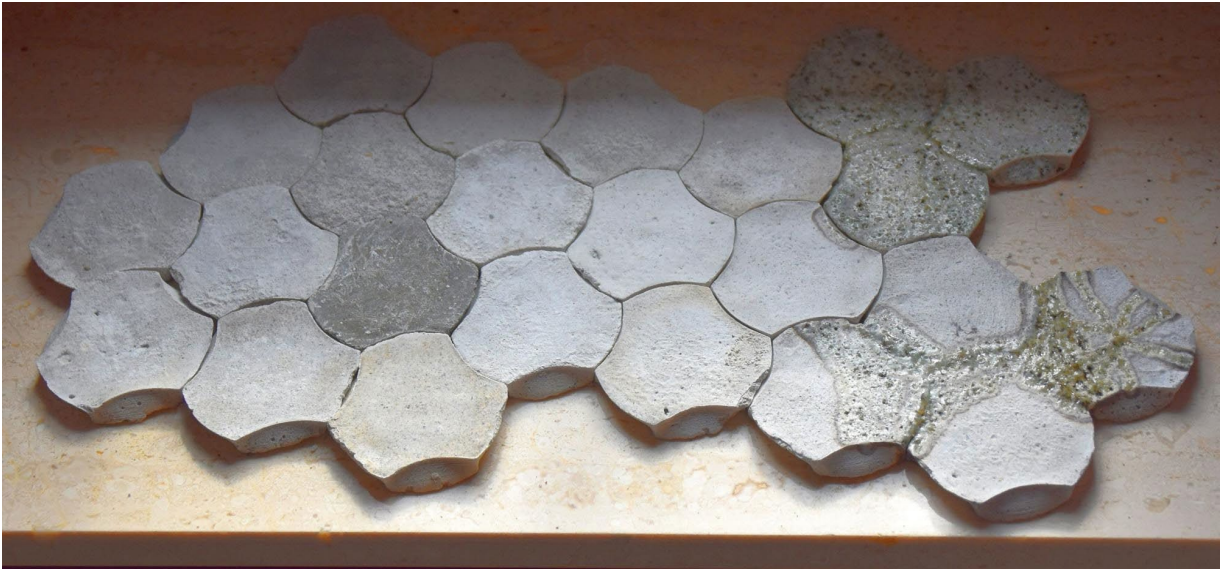
Geopolymer concrete tiles cast from >98% LSP-2 lunar highlands regolith simulant, using an interlocking tile mold of our design. The slabs on the right were vitrified and welded (!) with concentrated solar. Prepared by our collaborator Lucas Samuel in Belgium.
