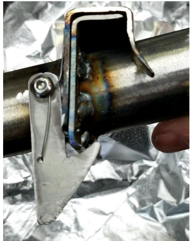
Welded steel prototype, which worked well, though it required quite a lot of hand welding.
