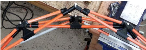
Scaled up origami design, composite rods with defined motion along 3D printed joints.
