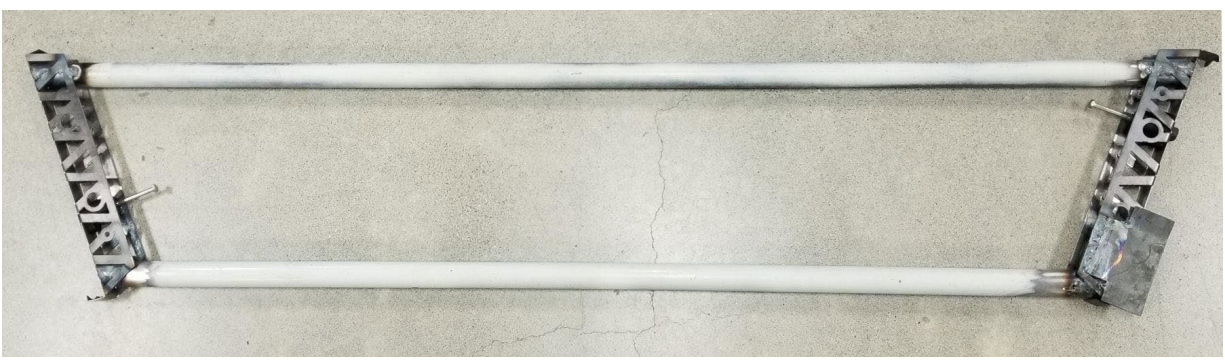
Upgraded plasma-cut endplate truss included an aligning feature, and locking pins.
