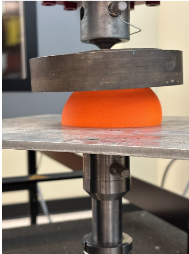
Figure 7-9: A Rock During the Compressive Test
