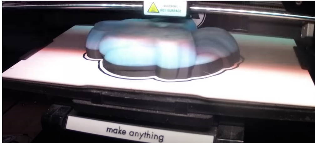
Figure 5-2: Climbing Handhold with Two Types of PLA
