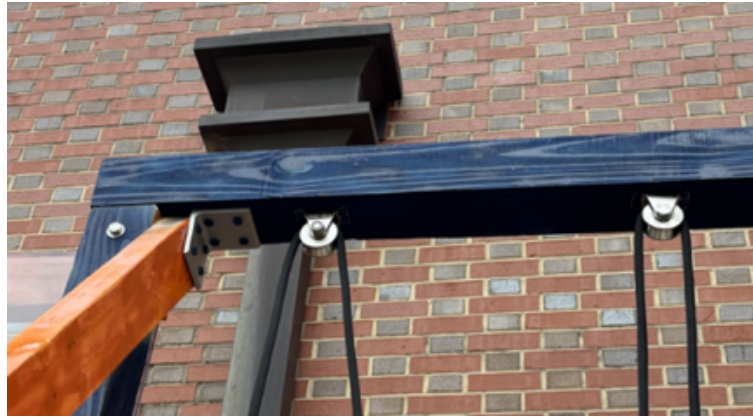
Figure 7-5: Pulley System for Bosun Chair
