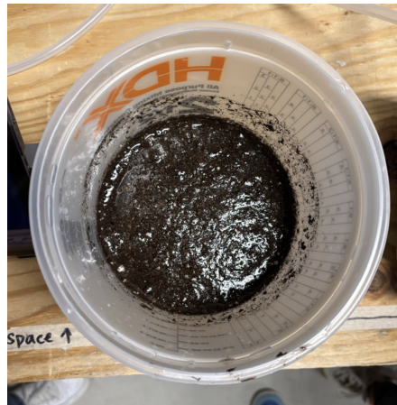
Figure 68: The 200 ml mixture containing 100 ml of sediment and 100 ml of water, which was replenished and used for all 3 trials
