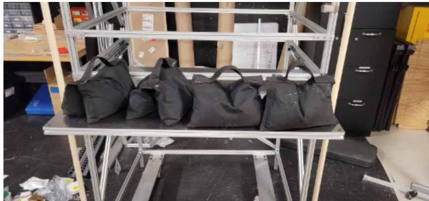
Figure 63: Desk Load Test
