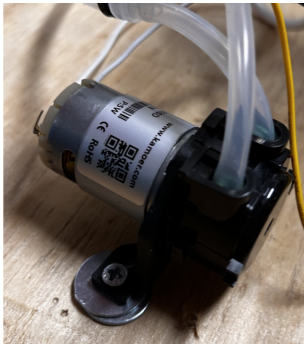
Figure 72: Pump Used For Feedwater Testing
