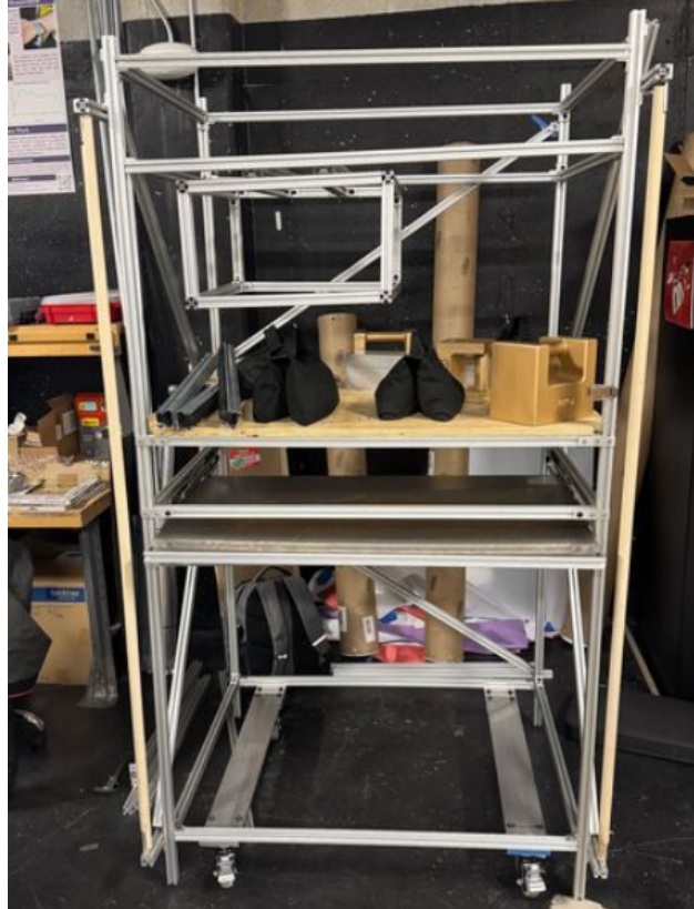
Figure 60: Rack Frame Load Test
