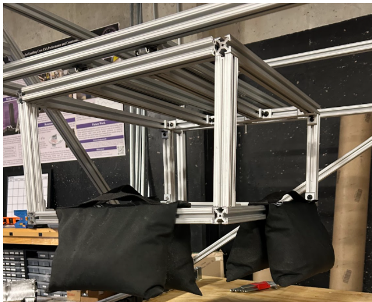
Figure 61: Load Testing Setup with Payload Pushed In
