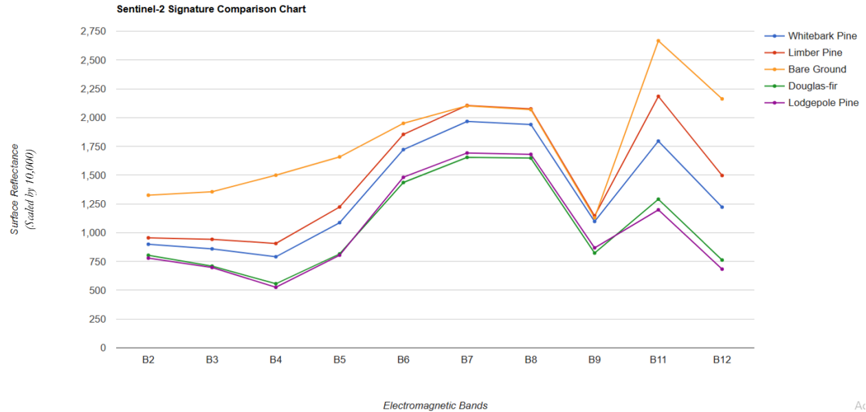
Figure 3. Spectral profile chart showing mean reflectance for each class at each Sentinel-2 band.
