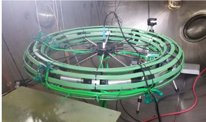
Figure 27. Magnetic field B_{00} calibration setup. High current cable leads can be seen on the vacuum tank floor. An array of 12 Faraday cups were positioned around the torus to collect the 600 eV protons from the ion beam.
