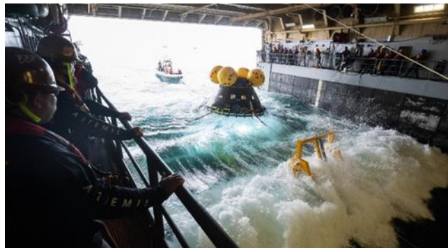
Figure 2 A wave breaks inside the well deck of USS Somerset as teams work to recover the Crew Module Test Article (CMTA), a full scale replica of the Orion spacecraft, as they practice Artemis recovery operations during Underway Recovery Test-12 off the coast of California, Thursday, March 27, 2025, NASA/Joel Kowsky 6 .
