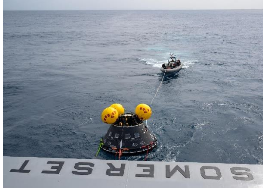
Figure 1 The Crew Module Test Article (CMTA). The CMTA is a full-scale mockup of the Orion spacecraft, is seen in the Pacific Ocean as teams practice Artemis recovery operations during Underway Recovery Test-12 onboard USS Somerset off the coast of California, Saturday, March 29, 2025. NASA/Bill Ingalls 6 .
