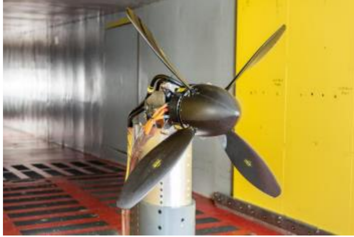
Fig. 2 Image of the test stand outfitted with the 36-inch diameter blades in the IRT [6].
