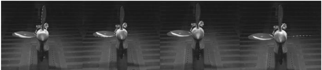
Fig. 11 Image series of the frames to receive the variance check input for the 36-inch diameter propeller assembly.
