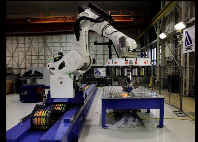
Multi-axis Automated Fiber Placement (AFP) Robot with in situ Inspection
