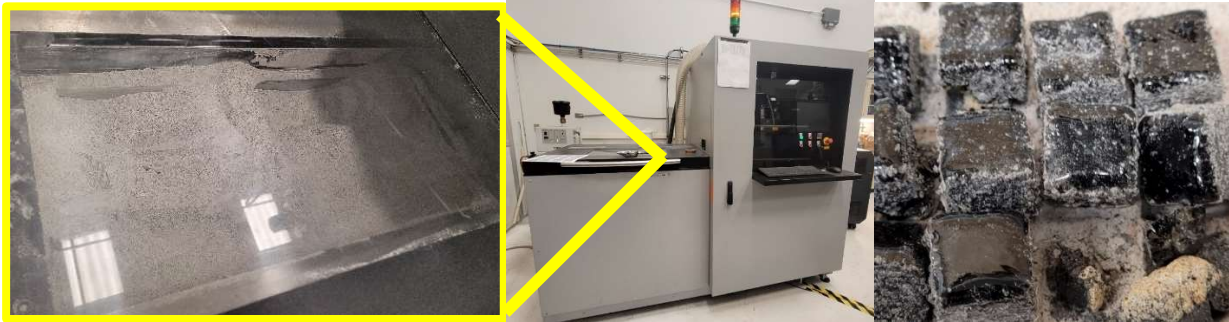
Fig. 4 Left: Modified LPBF printer filled with lunar regolith simulant (inset). Right: Close-up of highland regolith simulant parameter test cubes
