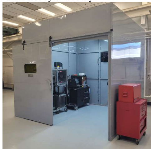
Fig. 11 Laser manufacturing cell for fast, safe development of laser processes and parameters, including integration into robotic systems.
