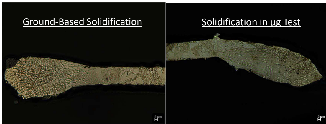
Fig. 8 Microstructure comparison of Inconel 625 solidification test foils
