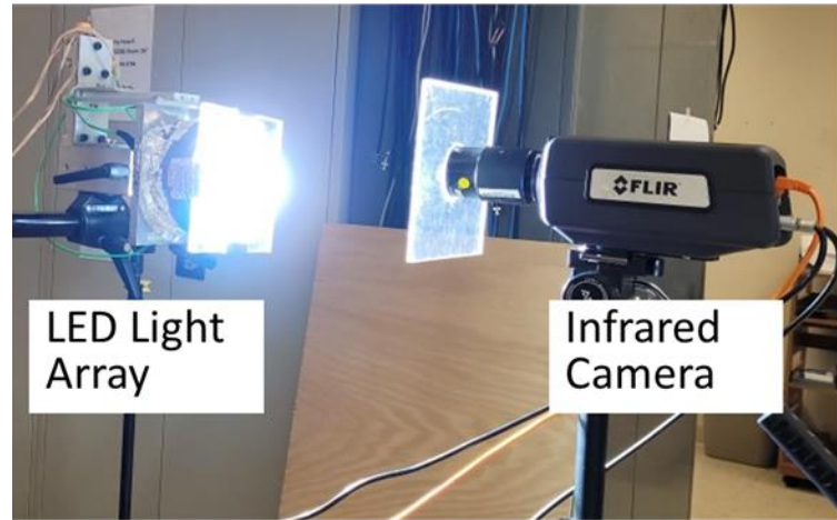
Direct View of Heat Source
