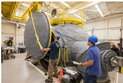
ESTA 15' TVAC Chamber with hatch closing
