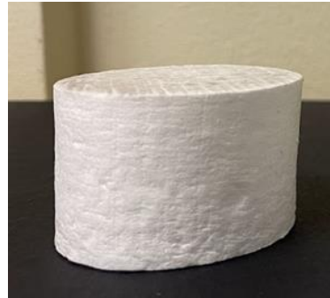
Sample = pure silica fiber billet made at JSC
