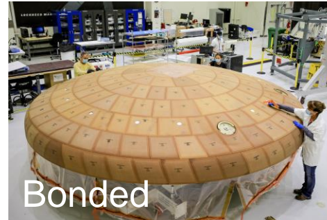
High-temperature Reusable Surface Insulation Tile Attachment System
