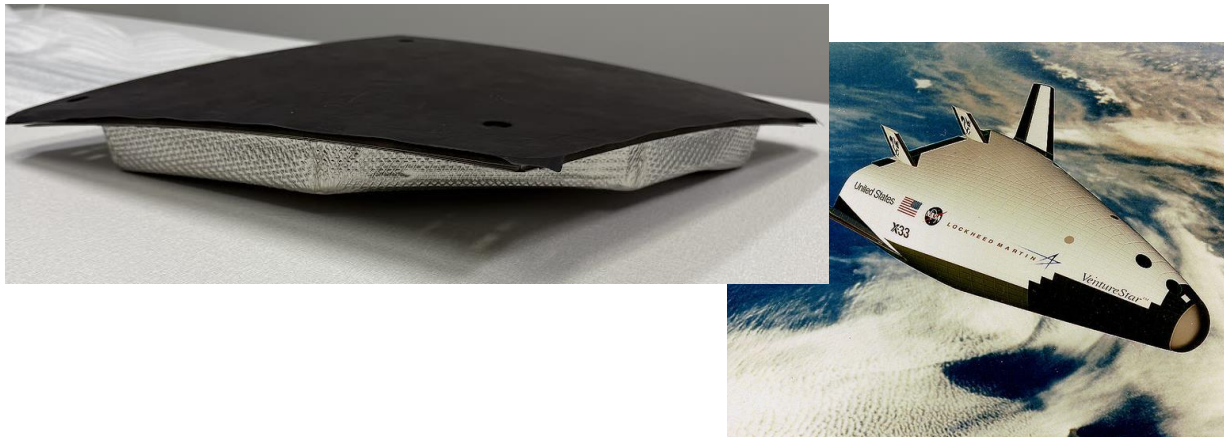
Figure 30. X-33 metallic TPS panel concept and attachment to the vehicle.
