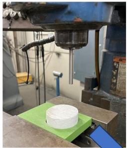
Using the cutting tool as sample holder in the mill
