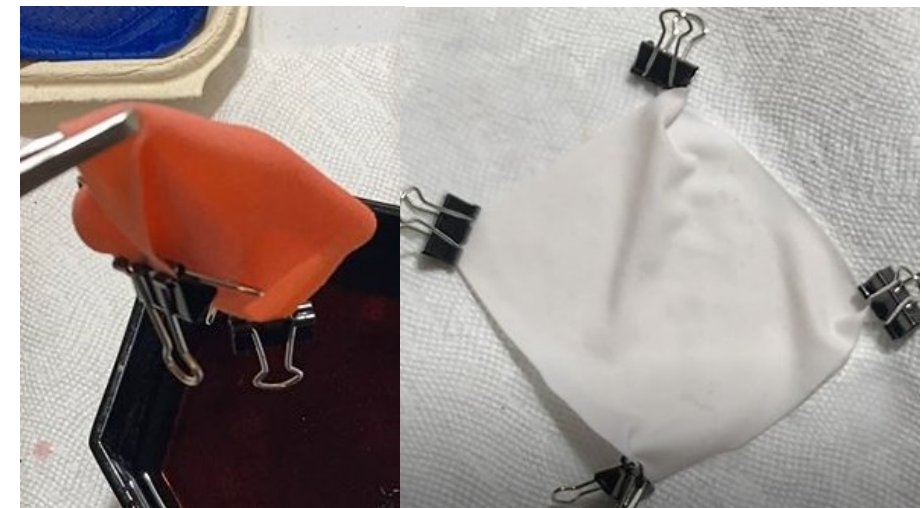
Dyed fabric after 3 min of Ultrasonic Cleaning before (Left) and after (Right) 7
