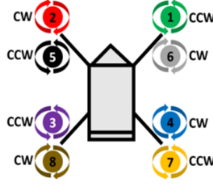
Fig. 7 Rotor numbering scheme used on the S-250 research vehicle and implemented in the CAMRAD II model.
