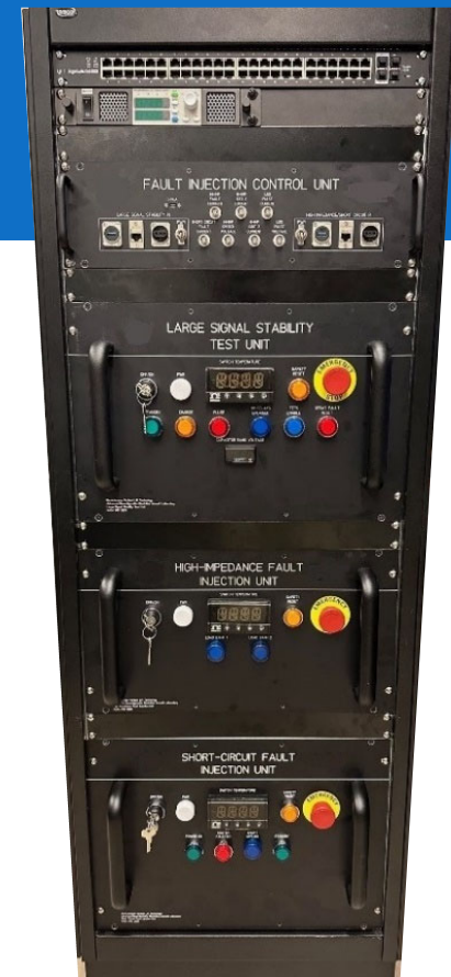
DC Fault Injection Unit
