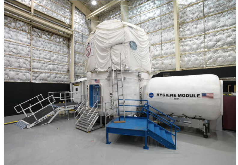
Human Exploration Research Analog (HERA), an isolation analog located at NASA Johnson Space Center that simulates future long-duration exploration missions
