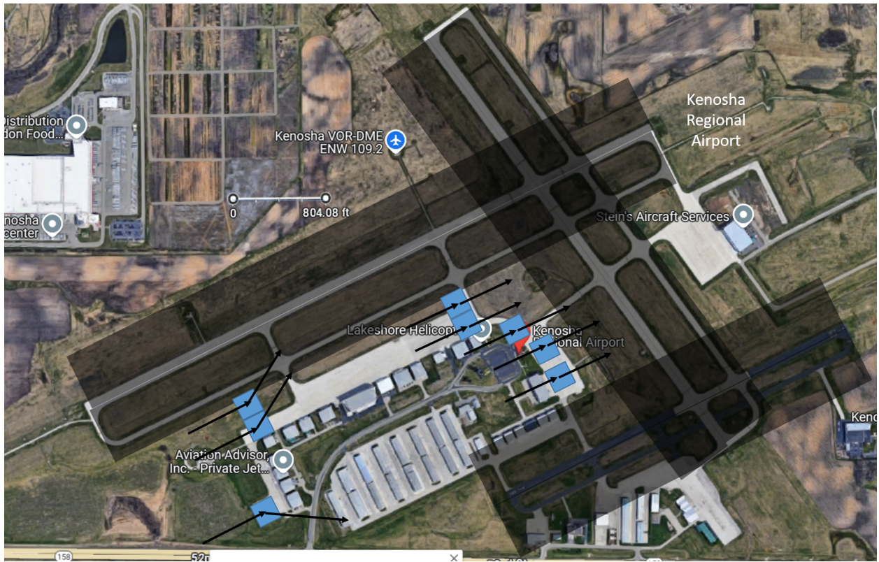
Fig. 8 TLOF pad locations for Kenosha Regional airport (KENW). Maps data: Imagery ©2025 Google, Imagery ©2025 Airbus, Maxar Technologies, Map data ©2025
