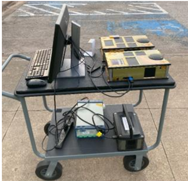
Figure 4: DITL live-sky testing of R5-S2 (upper right) and R5-S4 (center right)
