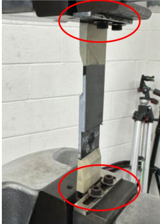
Figure 5.—L-brackets used to ensure alignment of SLS coupons during test.
