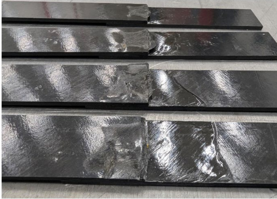
Figure 15.—Visual defects present on LM-PAEK induction-welded SLS coupons.
