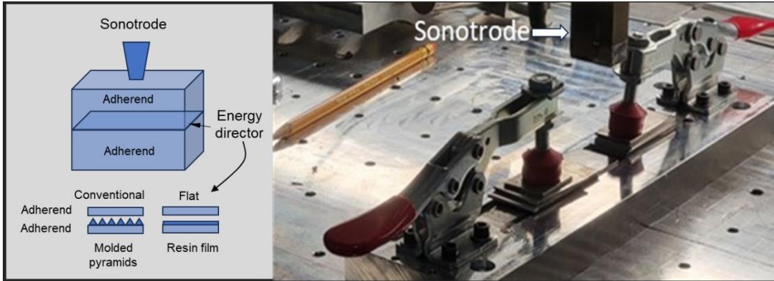
Figure 4.—Ultrasonic welding schematic and equipment used for this study.
