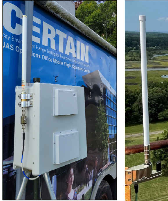
Figure 1-7. FLARM Sensor (left) and ADS-B Sensor (right) Installed on CERTAIN Range
