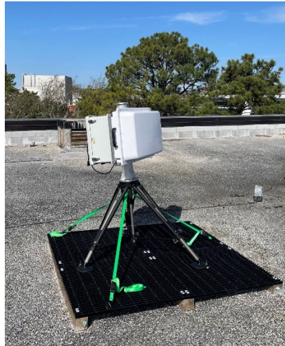
Figure 1-3. GA-9120 (w/SCM mounted on rear of radar) – Initial Field Setup
