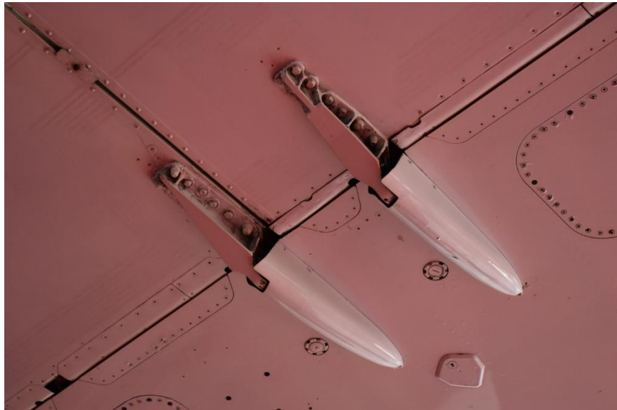
Figure 44- Example External Elevon Hinge Fairings (Aft Cover Removed, Mirage 2000)
