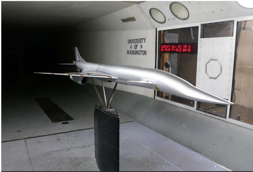
Figure 49- SCALOS Modular Model with RSAC Area-Ruled Body, Tested as “UW-S-24A”
