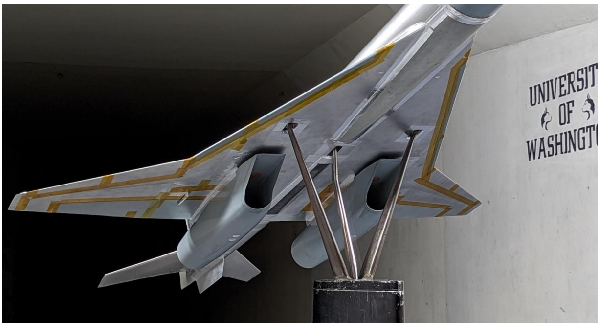
Figure 36- SCALOS N20 Nacelles in Bottom-Mounted (B) Location
