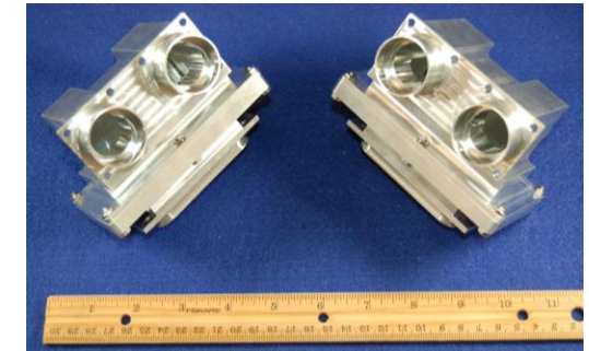
A pair of Gen-2 TCC canisters developed for low pressure drop & integration with a CO 2 /H 2 O removal module
