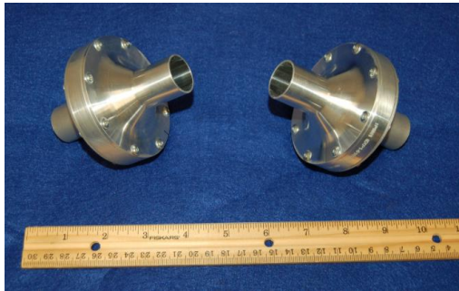
A pair of Gen-1 TCC canisters developed for vacuum-swing operation (used for sorbent evaluation/development)
