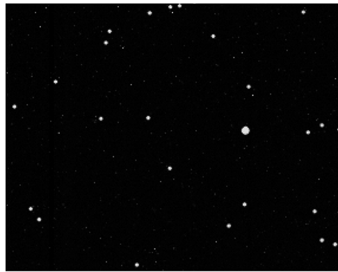
Figure 7. A subregion of an image captured during a beam spill. Note that an individual ion's generated charge may be collected within an individual pixel or across clusters of pixels.
