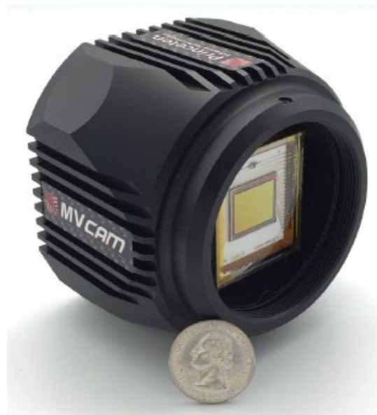
Figure 1. Picture of the 1280MVCam in a standard package. The camera that was evaluated during this test campaign had a custom aluminum enclosure.
