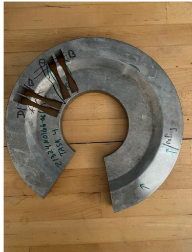
Starting material of wrought (pictured), flow-formed Al2195, and flow-formed Al6061
