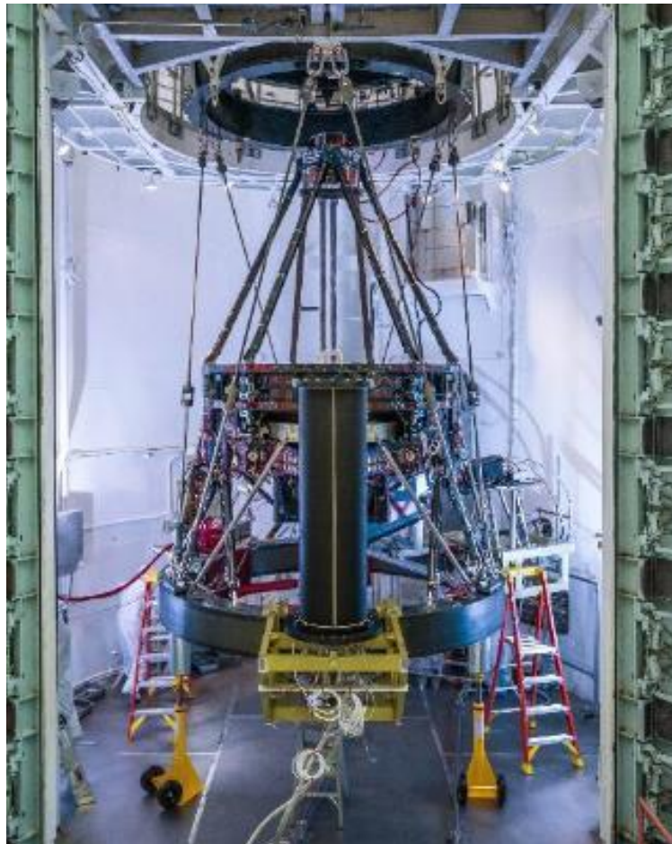
Figure 4 IOA in test chamber. CGI test equipment in front center, WFI test equipment in right rear.
