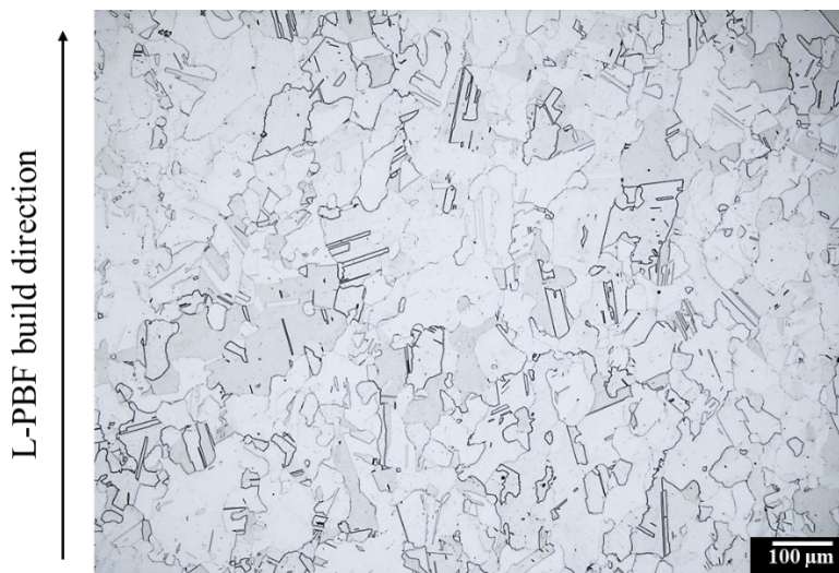
Figure 30. The typical microstructure (in X-Z plane) of L-PBF NASA HR-2 specimen used for tensile testing in 5-ksi \text{GH}_2 environment. The average grain size is approximately 75 \mu\text{m} .
