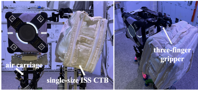
Fig. 3. Astrobee grasping an single-size ISS CTB with the three-finger gripper prototype while free-flying on the granite table.
