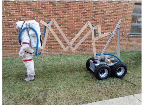
Figure 21. Passive pantographic umbilical handling mechanism
