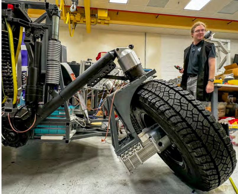
Fig. 22 The steering actuators integrated between the swingarm and the wheel structure, with the caster adjustment bar and pin-hole structure to the left. Wheel drive wiring pass externally with slack to allow steering rotation.
