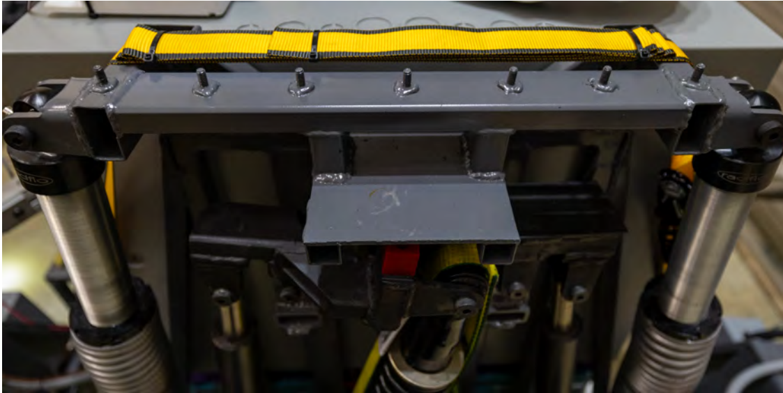
Fig. 28 Weld studs added atop the suspension
