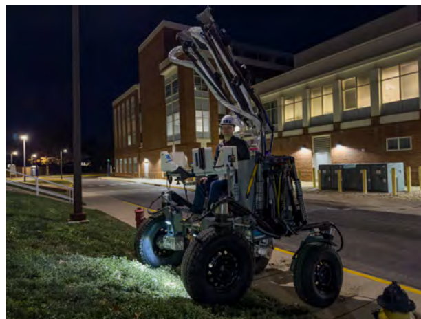
Fig. 45 Complete VERTEX with ARMLiSS climbing the 21° hill
