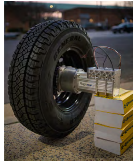
Figure 18. Wheel Assembly Test Fit
