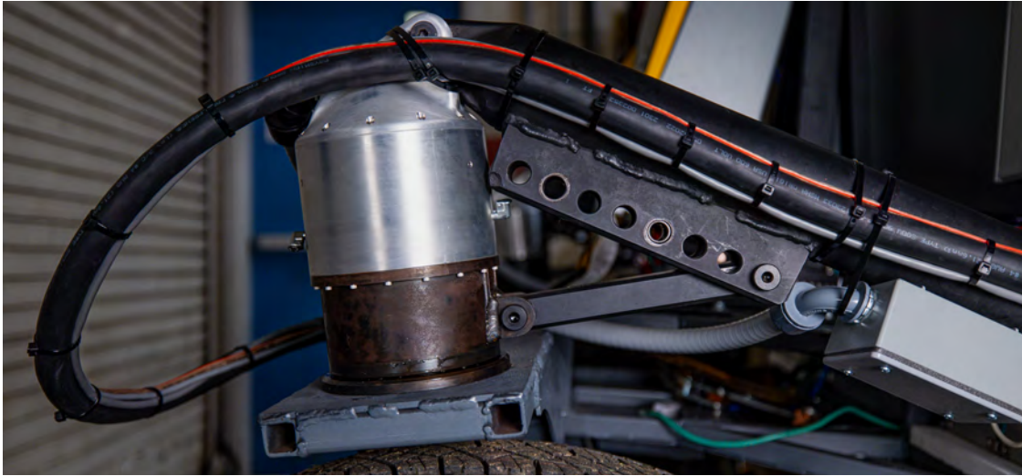
Fig. 34 Caster adjustment mechanism side profile
