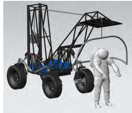
Fig. 27 Corner view of astronaut mass offset concept
