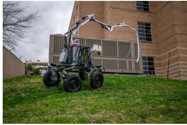
Figure 20. Additional angle of BioBot with ARMLiSS fully extended on slope
