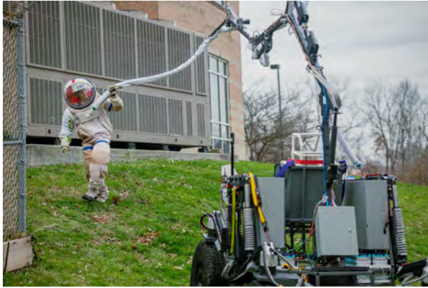
Fig. 51 Slope testing with ARMLiSS fully extended
