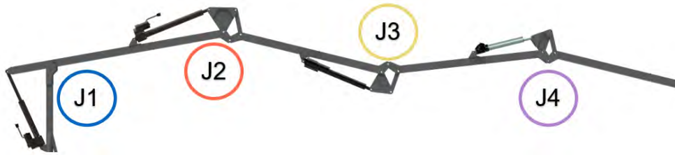
Fig. 8 Diagram of arm joint locations, corresponding to torques in Fig. 9. Structural links are numbered by their proximal joint, with the vertical mast being link 0 and the tip being link 4.
