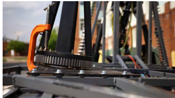
Fig. 22 Deflection in BioBot arm mounting plate
