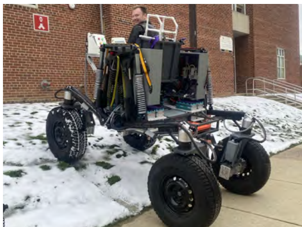
Fig. 44 First full integration tests climbing a 21° hill
