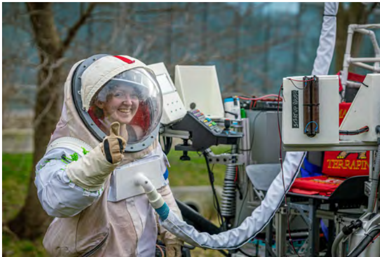
Figure 7. Closeup of MX-C+ suit with umbilical attachment and FDM printed bearing arm
