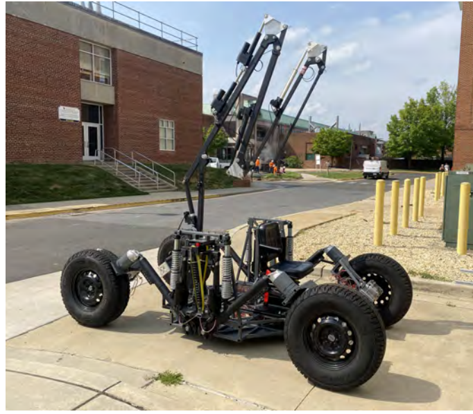
Fig. 11 Retracted ARMLiSS integrated with the kneeling VERTEX rover, clear of the driver for ingress.
