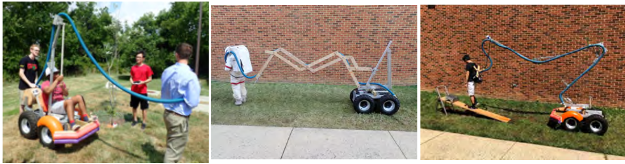
Figure 2. Phase 1 preliminary designs: (L-R) single point catenary design, pantograph-type kinematic chain design, and actively-controlled manipulator[2].
