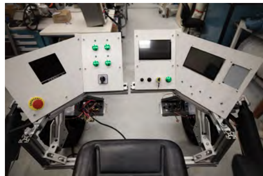
Figure 28. Integrated control panel in closed position
