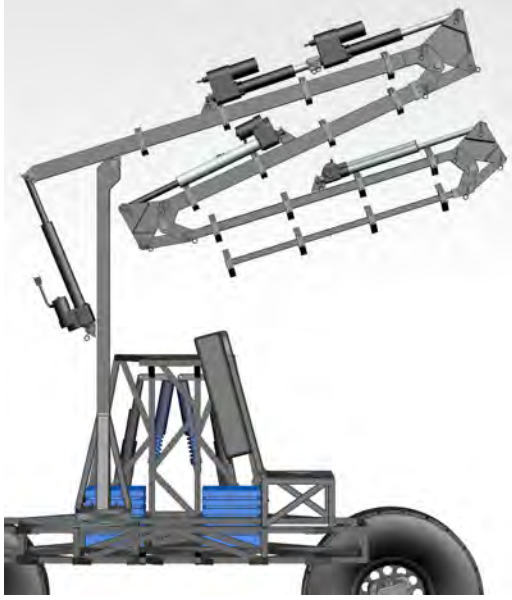
Fig. 10 Umbilical arm in its retracted "stowed" pose, mounted on a cross-section of the VERTEX rover.
