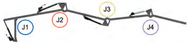
Figure 4. Diagram of arm joint locations, corresponding to torques in Fig. 5. Structural links are numbered by their proximal joint, with the vertical mast being link 0 and the tip being link 4.
