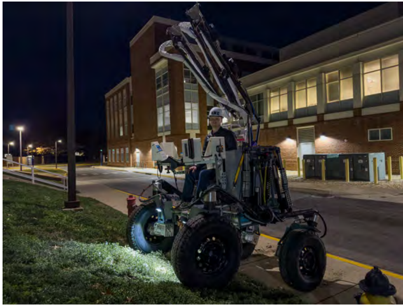
Figure 11. Full BioBot system climbing a hill for the first integrated test
