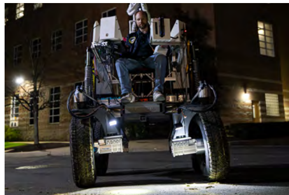
Fig. 35 Camber differential shown on front two wheels during a test
