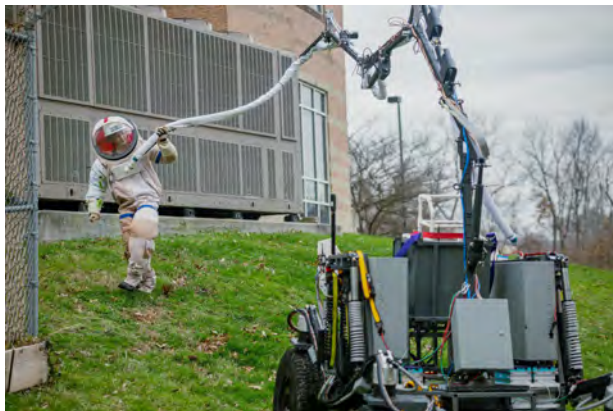
Figure 17. Slope testing with ARMLiSS fully extended
