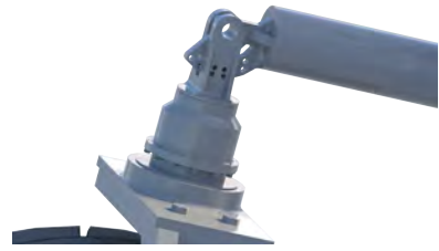
Figure 13. VERTEX's manual caster adjustment mechanism
