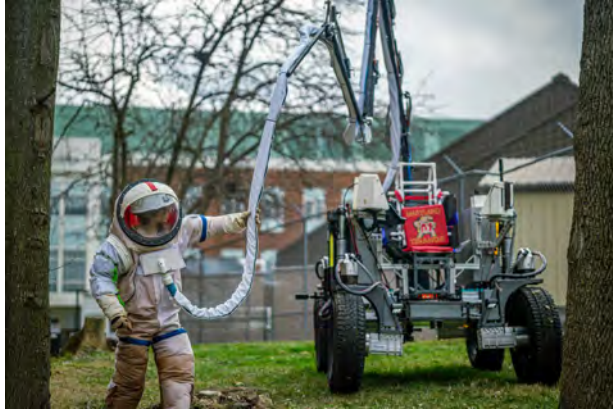
Figure 15. Test subject manually moving umbilical arm around VERTEX
