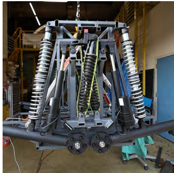
Figure 4. VERTEX suspension with series-elastic linear actuators
