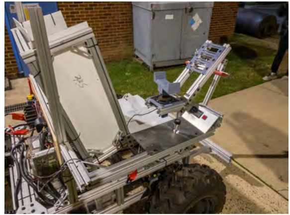
Figure 8. RAVEN rover outfitted with conceptual controllers for initial position and accessibility tests
