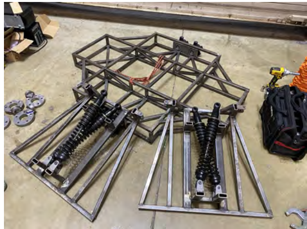
Fig. 27 Finished chassis walls with suspension 1 configuration
