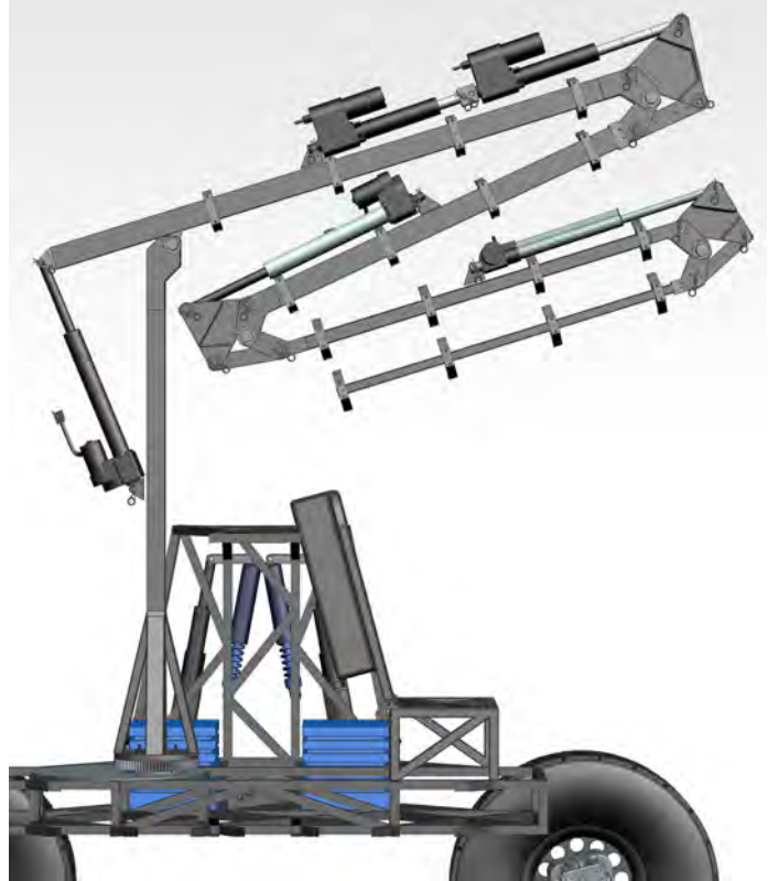
Figure 9. Umbilical arm in its retracted "stowed" pose, mounted on a cross-section of the VERTEX rover and ready for astronaut driving.
