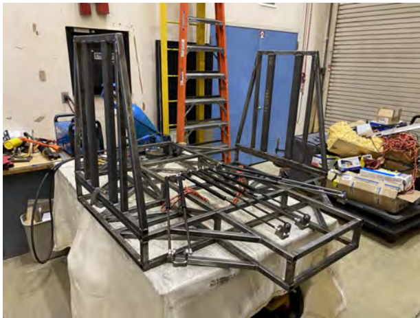
Fig. 26 Chassis wall preliminary assembly with chassis
