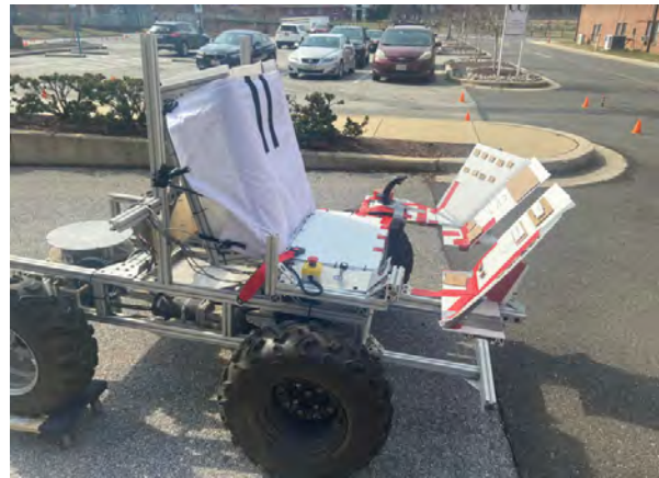
Figure 11. RAVEN with the control panel and seat mockups
