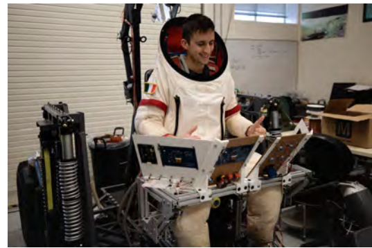
Figure 30. Integrated control panel in closed position with test subject
