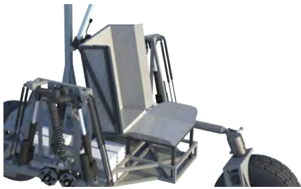
Figure 31. Bent sheet steel and welded seat chassis concept
