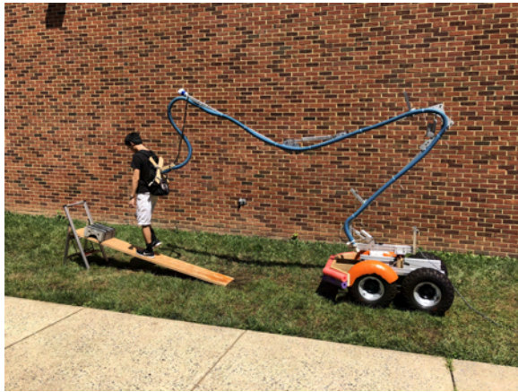
Figure 20. Actively controlled robotic umbilical handling mechanism
