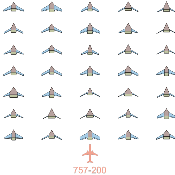
Figure 7: DOE geometry output and down select to useful planforms
