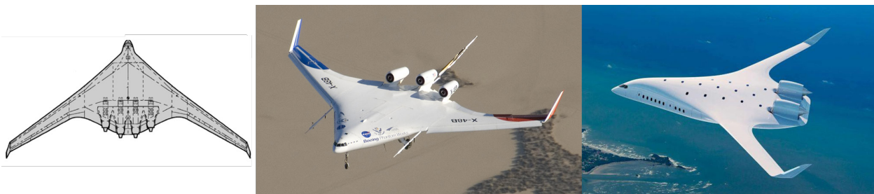
Figure 2: Early McDonnell Douglas BWB design, Boeing X48B demonstrator, and JetZero airliner rendering
