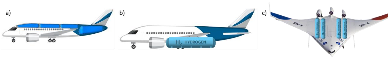
Figure 2. The possible locations of LH_2 storage for commercial transport aircraft are a) inside the fuselage, b) suspended over the wing, or c) in a new blended wing body design.
