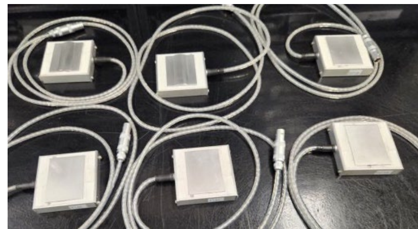
Prototype sensors (2 curved front & back, 2 flat front, curved back, 2 flat front & back)
