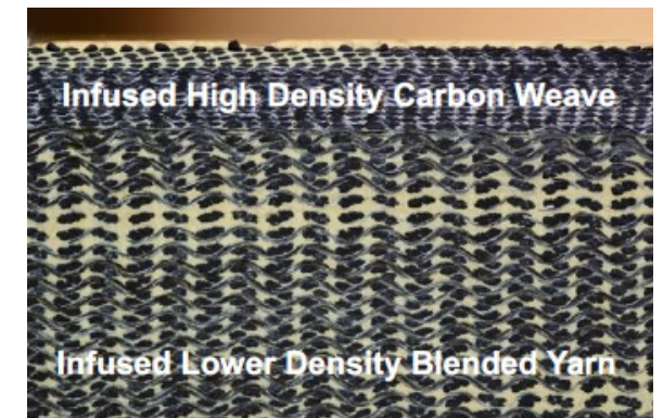
Infused 3D weave microstructure
