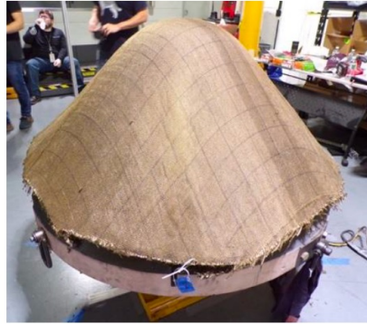
Formed and trimmed sphere-cone preform
