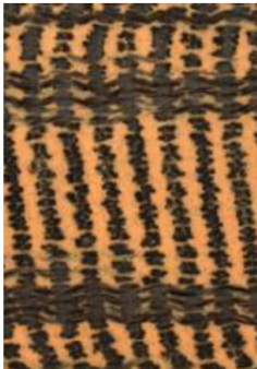
Variability in yarn stacking during weaving process
