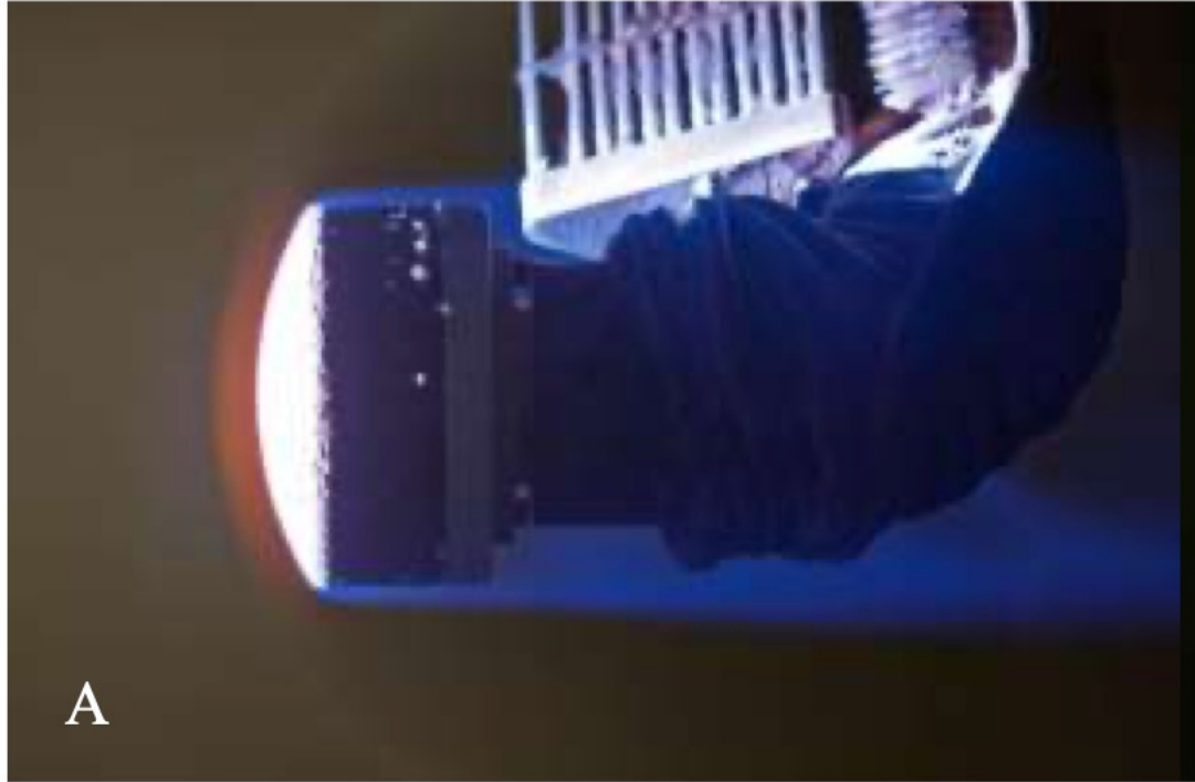
Martian regolith-RTV in the Arc Jet
