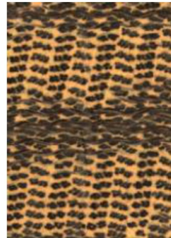
Variability in yarn stacking during weaving process
