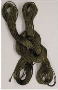
Twisted and stretch-broken yarn
