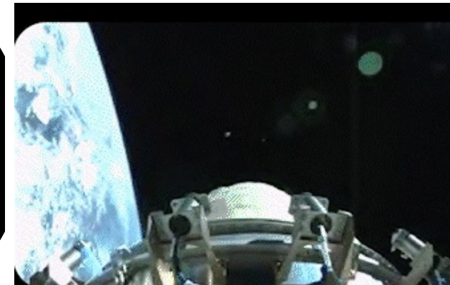
LOFTID deployment before entry. NASA
