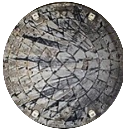
Artemis I Avcoat heat shield. NASA
