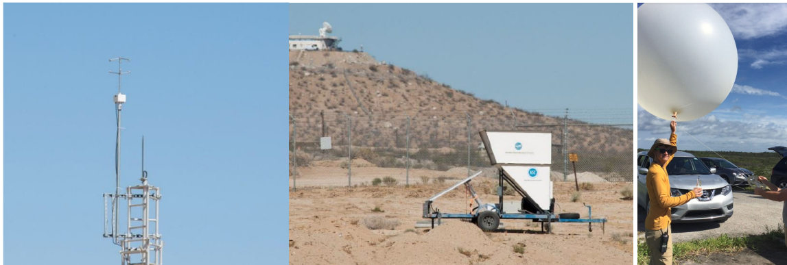
Figure 4. Meteorological measurement equipment from the SonicBAT flight test. Left: sonic anemometer. Center: SODAR. Right: weather balloon. Left and center photos were adapted from Ref. [6].
