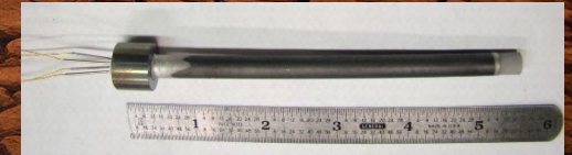
Resistive SiC pressure sensor in preparation for evaluation in GEER.
