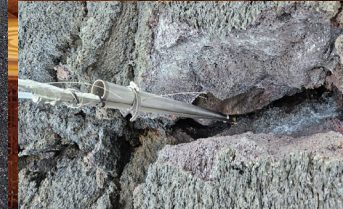
Chemical Sensor Probe Suspended in Lava Surface Crack
