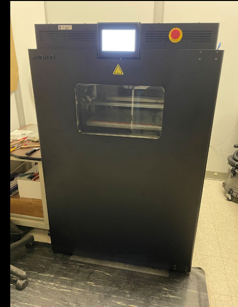
AON M2+ PEEK, PEKK, ESD Polycarbonate Build Volume: 450 × 450 × 565 mm
