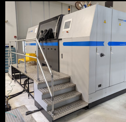
Concept Laser Xline 2000R In718 Build Volume: 400 x 800 x 500 mm
