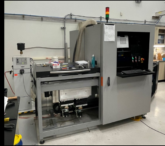
Laser Fusion Solutions upgraded M1 Various Materials including Lunar Regolith Simulant Build Volume: 250 mm 3
