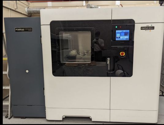
Stratasys Fortus 900 ABS, Polycarbonate, Ultem 9085, Antero 840CN03 Build Volume: 914 x 609 x 914 mm
