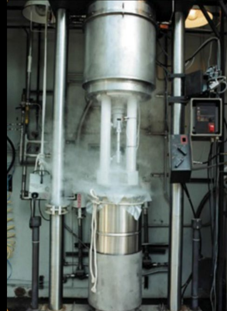
Tension Test in Liquid Hydrogen
