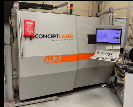
Concept Laser M2 GRCo-42 Build Volume: 245 x 245 x 350 mm
