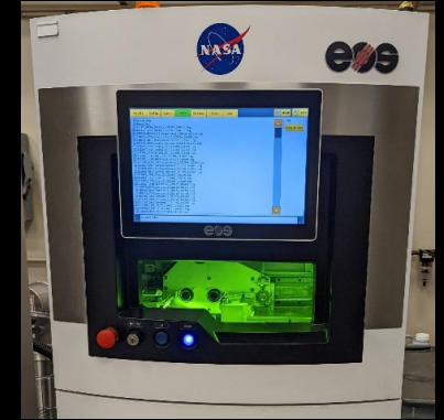
EOS M100 Various Materials Build Volume: 100 \phi x 95 mm z
