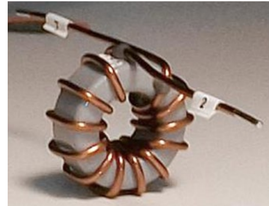
Classic toroid power inductor, for Space
