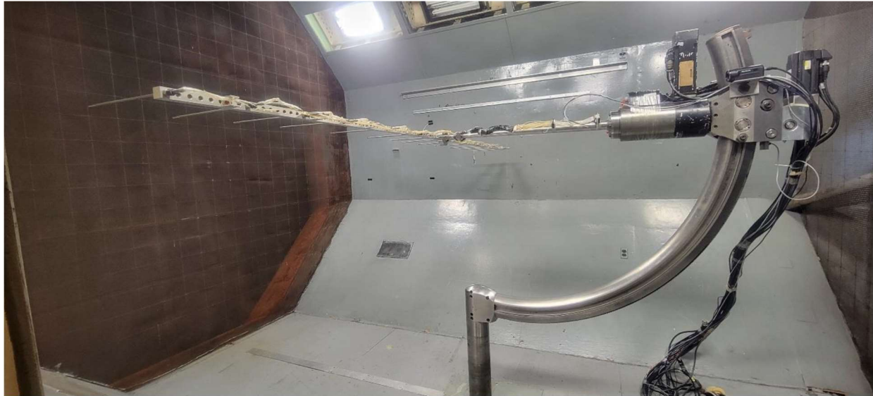
Figure 5 – Flow survey rake attached to the roll oscillation rig on the C-Strut.
