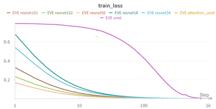
Figure 10. Training loss curves comparing various baseline models (ResNet18, ResNet34, ResNet50, ResNet101, ResNet152, UNet, and Attention UNet) for the Solar EUV irradiance prediction task. UNet and Attention UNet show slower initial convergence compared to ResNet variants but achieve significantly lower final loss values, highlighting their effectiveness in modeling complex spatial patterns inherent to solar EUV spectra.
