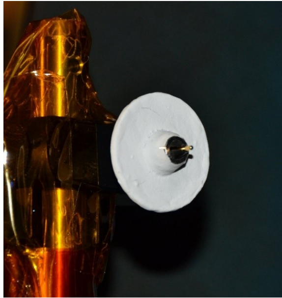
Figure 4: Custom-built reference target for in-situ laser alignment [20].
